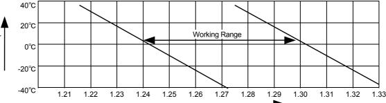
Specific gravity of battery fluid
